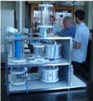
Within a QREN/Compete project, researchers from CERENA/ISEL were able to develop a process producing methane from renewable electricity. A prototype of 1 kW is currently under test in ISEL laboratories.
